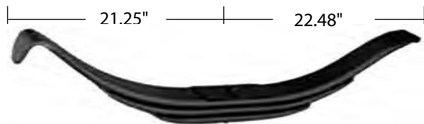
Trailer Spring, Three Leaf - High 5 1 / 2 " Arch Heavy Duty - 24,000 lb. GAWR Interchanges TRA-2740 Part No. 365-00
